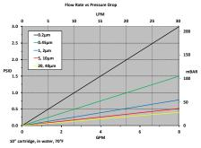
$^*\!All$  data is based on absolute rated medias. Nominally rated medias will result in a pressure drop reduction of approximately 10%.
